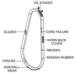
Figure 7. Drive Belt Inspection
